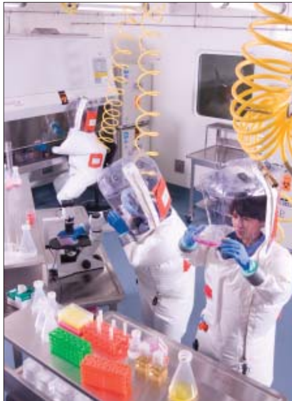
When researchers are wearing the Shope lab’s “space suits,” even routine lab procedures require special care. One researcher compares being in the suits to “working inside a big plastic bubble.” The hoses dangling from the lab’s ceiling provide air for breathing and to keep the suits pressurized.
